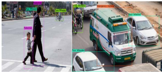
Fig 7: Detection and classification by our trained YOLOv4 Model
